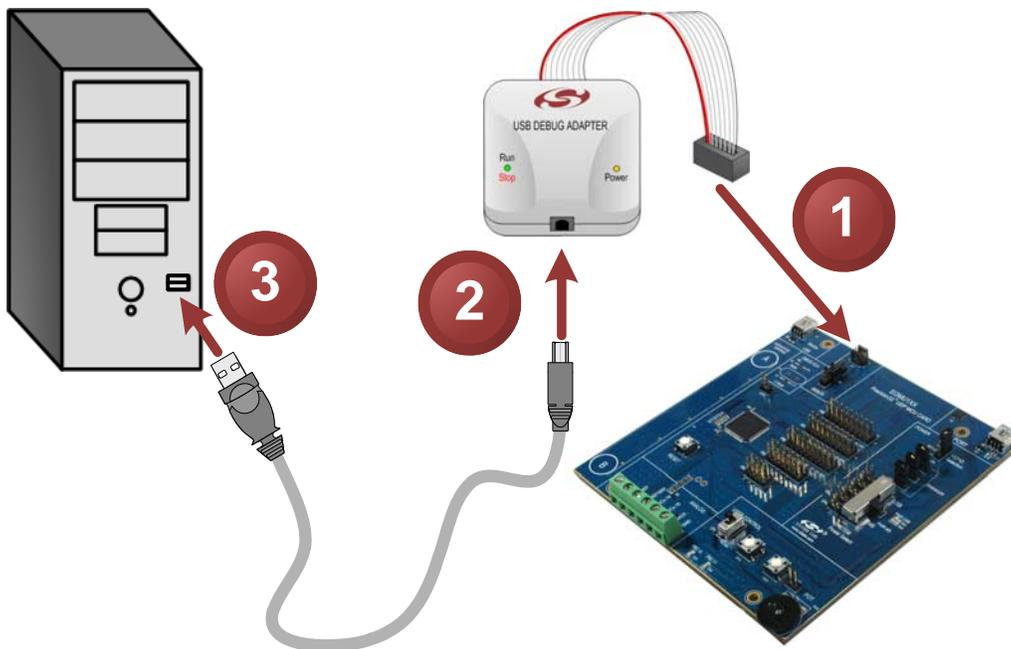
Figure 3. Hardware Setup using a USB Debug Adapter
