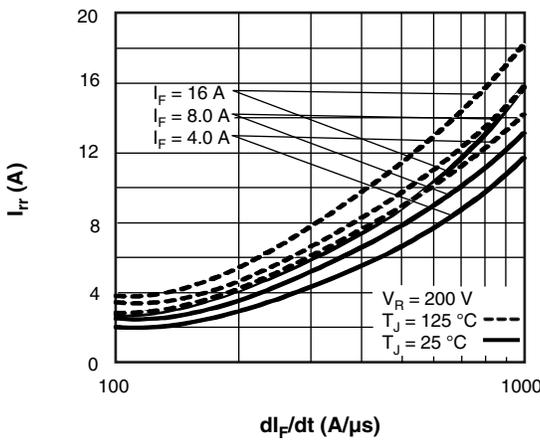
Fig. 6 - Typical Recovery Current vs.  $di_F/dt$  (Per Leg)
