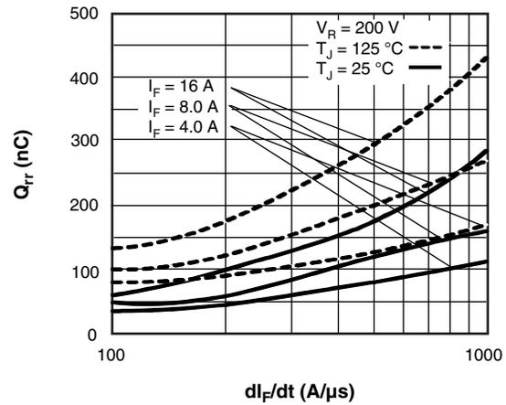
Fig. 7 - Typical Stored Charge vs.  $di_F/dt$  (Per Leg)
