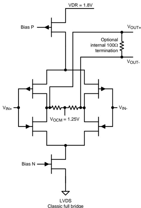
Figure 18. Output Driver Circuit: LVDS
