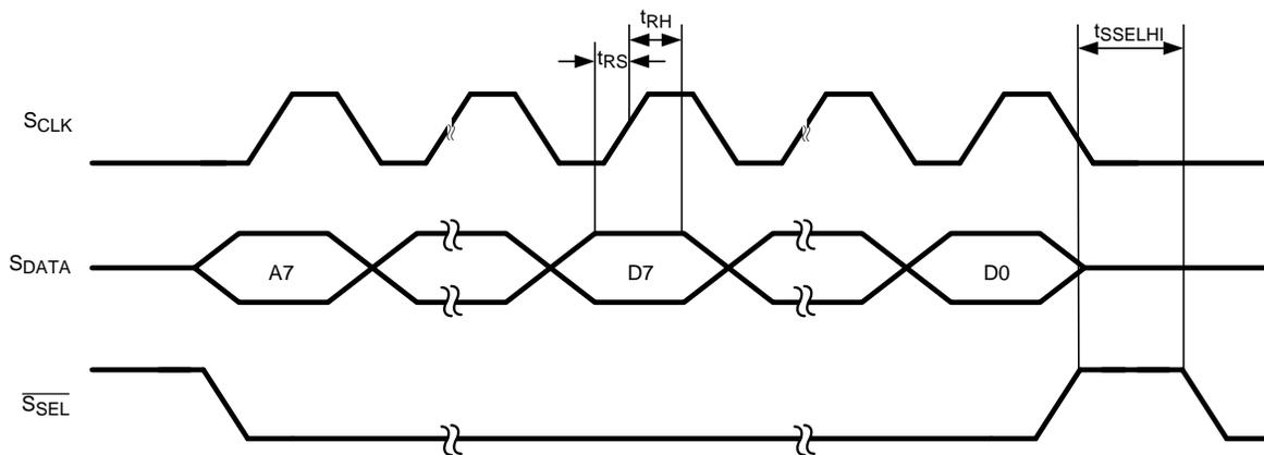
Figure 5. SPI Read Timing
