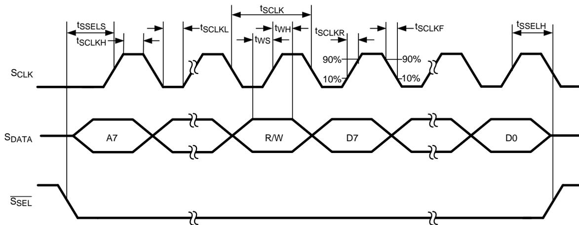
Figure 4. SPI Write Timing
