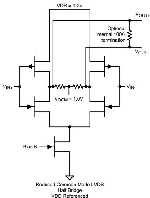
Figure 17. Output Driver Circuit: Reduced Common Mode LVDS
