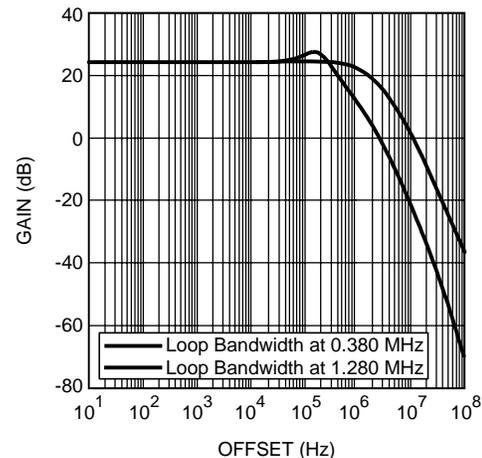
**Figure 13. PLL Phase Noise Transfer Function:  $f_s = 50\text{MHz}$**
