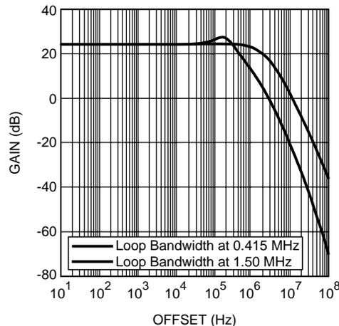
**Figure 12. PLL Phase Noise Transfer Function:  $f_s = 40\text{MHz}$**
