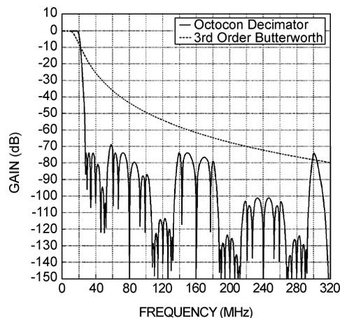
Figure 9. Digital Filter Transfer Function
