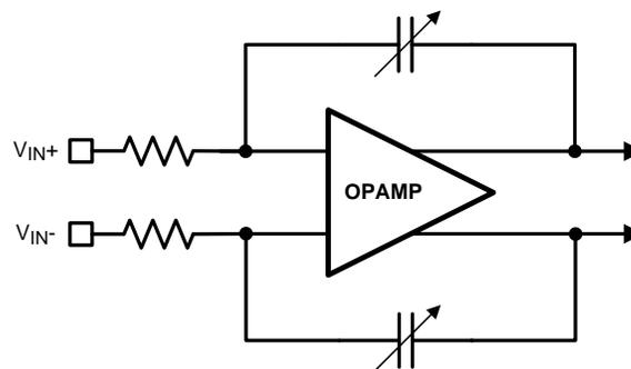
Figure 7. Continuous Time Sigma Delta Input Stage
