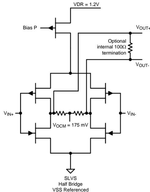
**Figure 19. Output Driver Circuit: SLVS**
