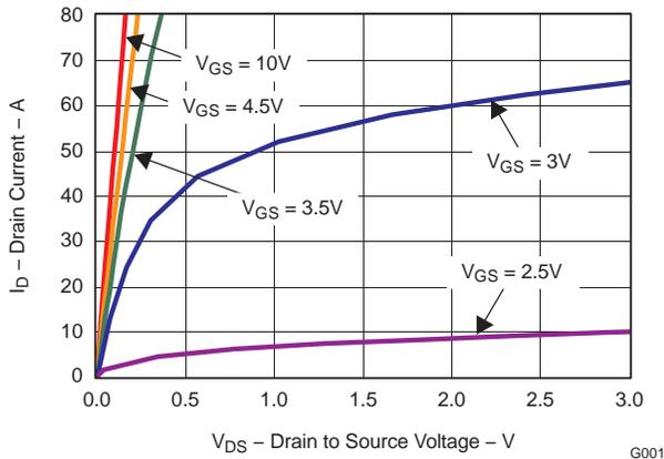
**Figure 2. Saturation Characteristics**
