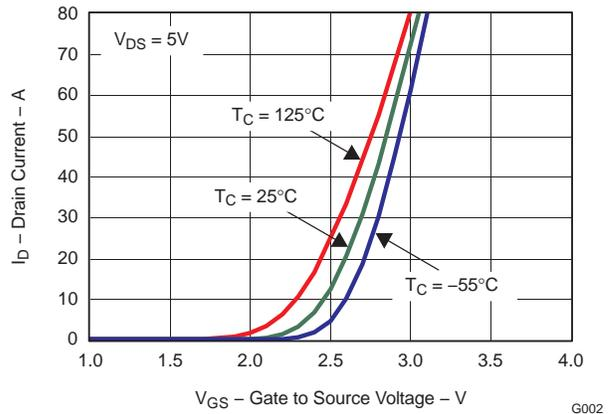
**Figure 3. Transfer Characteristics**
