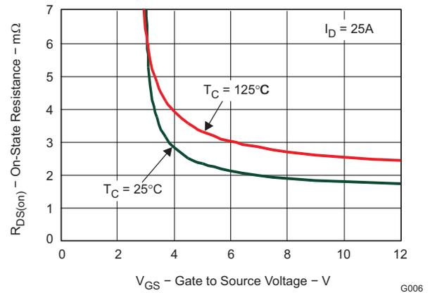
**Figure 7. On-State Resistance vs. Gate to Source Voltage**
