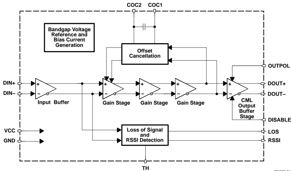
Figure 1. Simplified Block Diagram of the ONET4251PA
