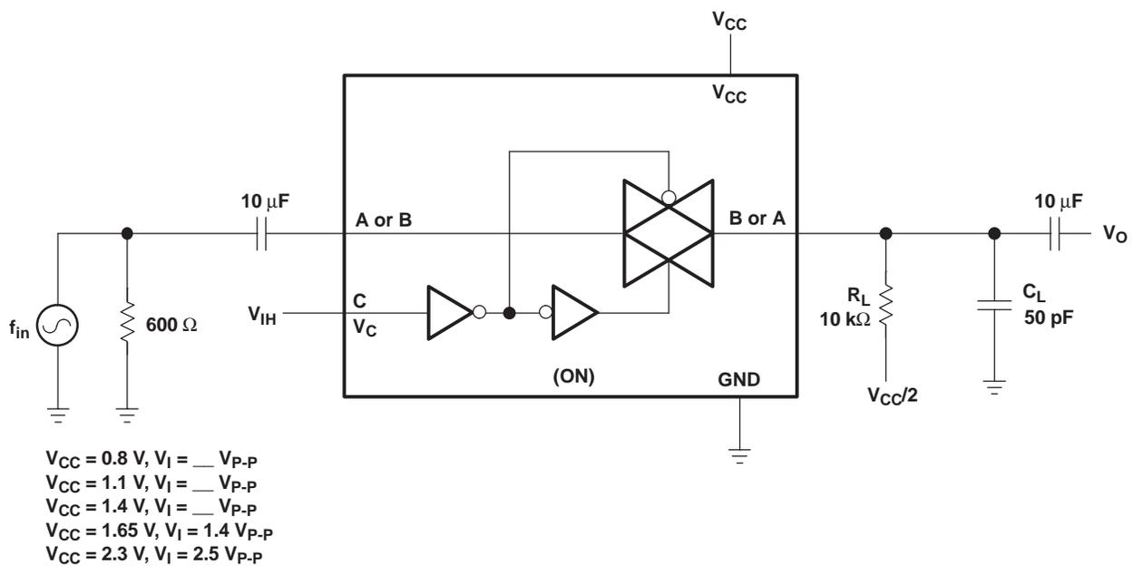
Figure 8. Sine-Wave Distortion
