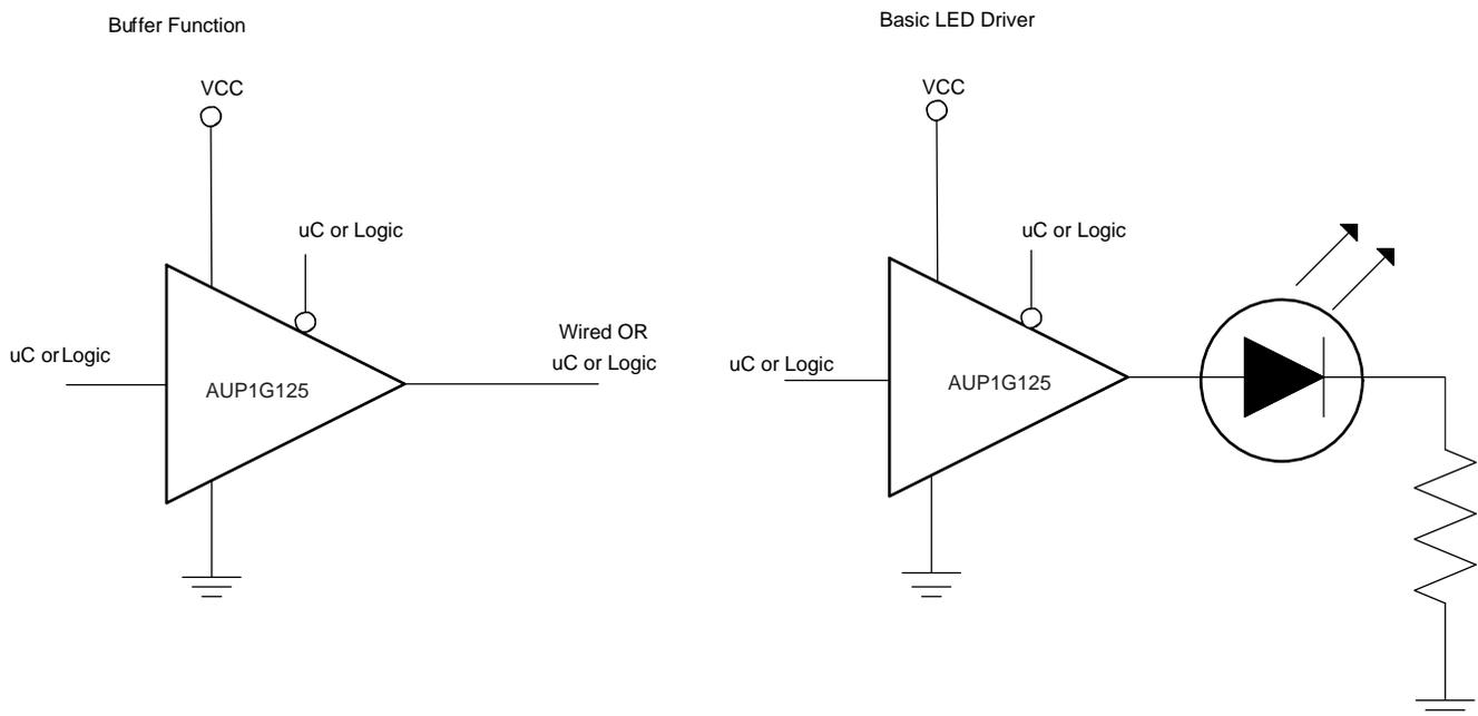
**Figure 4. Application Schematic**
