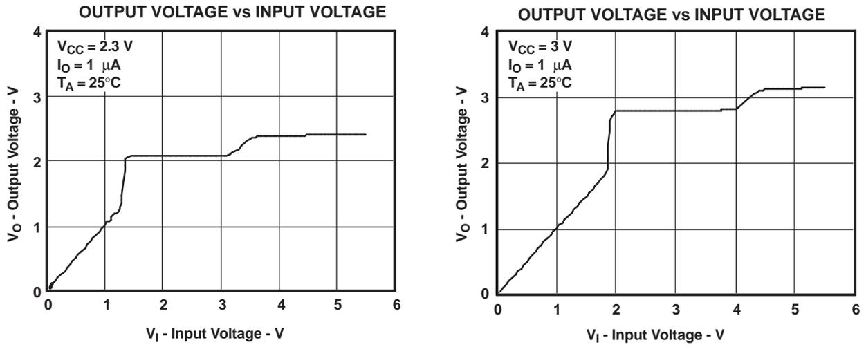
Figure 3. Data Output Voltage vs Data Input Voltage
