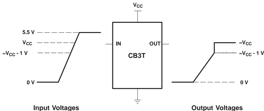
If the input high voltage ( $V_{IH}$ ) level is greater than or equal to  $V_{CC} - 1V$ , and less than or equal to 5.5V, the output high voltage ( $V_{OH}$ ) level will be equal to approximately the  $V_{CC}$  voltage level.
