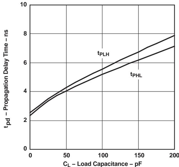
NOTE: This graph is included as an aid to the system designers. Total circuit delay varies with load capacitance. The total delay is the sum of the delay due to external capacitance and the intrinsic delay of the device. Intrinsic delay is listed in the table above as the 0 pF load condition. The incremental increase in delay between the 0 pF load condition and the actual total load capacitance represents the extrinsic, or external delay contributed by the load.
