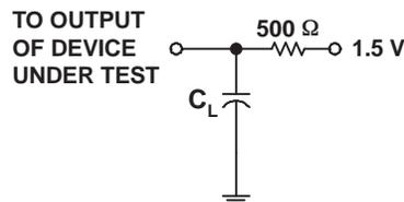
Figure 9. Receiver Disable Time ( $t_{PHZ}$ ,  $t_{PLZ}$ ) Test Circuit
