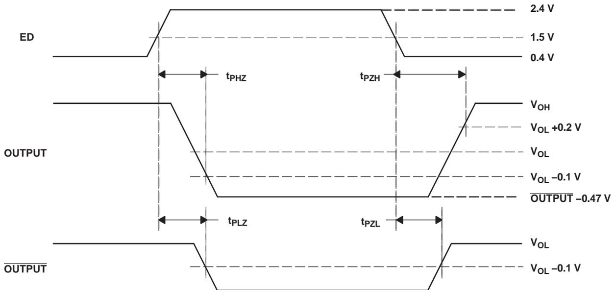
A. NOTE: In the third state, OUTPUT is 0.47 V (minimum) more negative than  $\overline{\text{OUTPUT}}$ .
