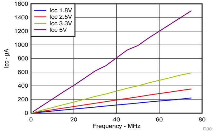
Figure 5. I<sub>CC</sub> vs Frequency
