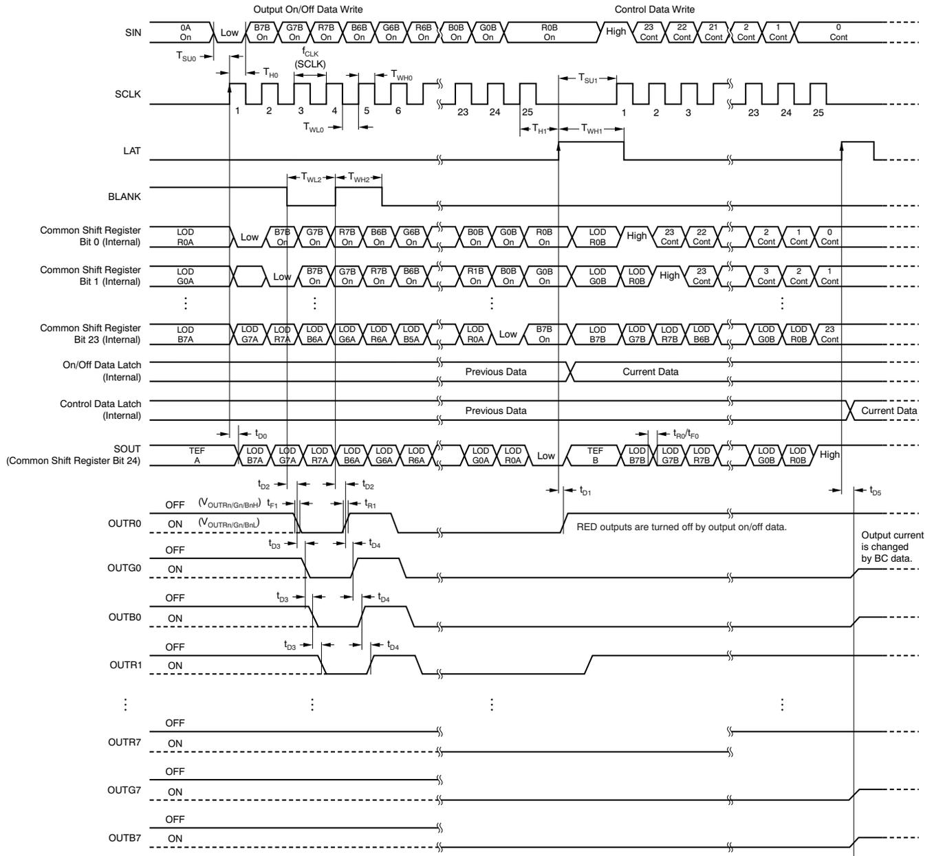
**Figure 9. Timing Diagram**
