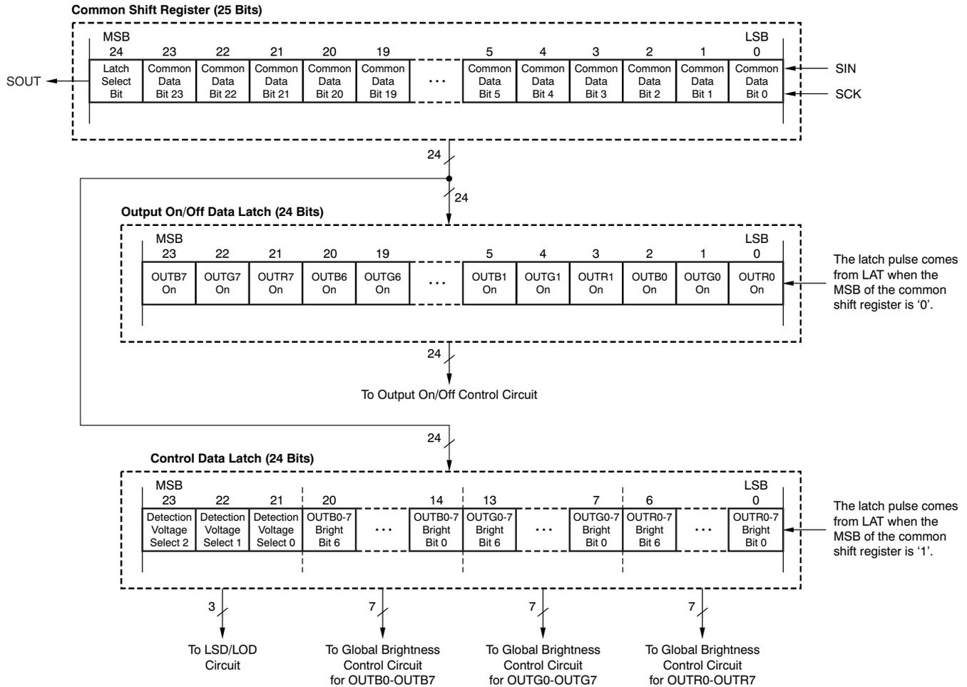
Figure 33. Grayscale Shift Register and Data Latch Configuration
