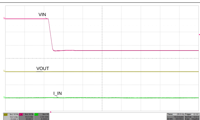
Figure 63. Reverse Polarity Protection
