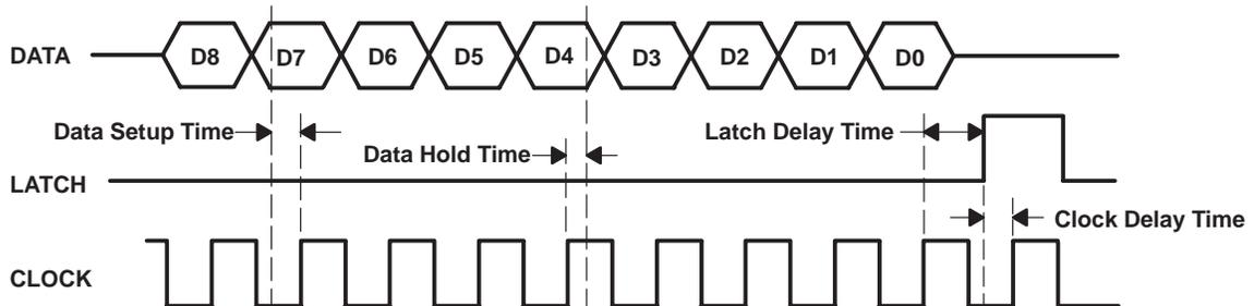
NOTE: Data is clocked in on the positive edge of the clock. The positive edge of the latch signal should occur before the next positive edge of the clock. For definition of D0 to D8, see the control logic table.
