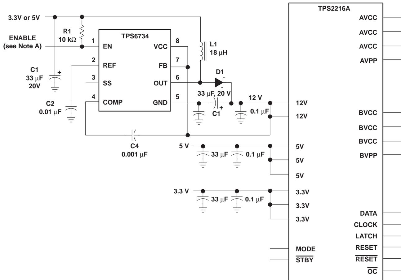
NOTE A: The enable terminal can be tied to a general-purpose I/O terminal on the PCMCIA controller or tied high.
