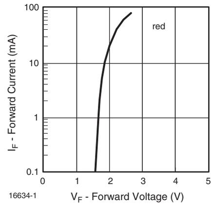
Fig. 4 - Forward Current vs. Forward Voltage
