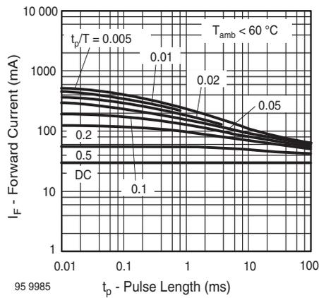
Fig. 2 - Pulse Forward Current vs. Pulse Duration
