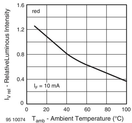
Fig. 5 - Relative Luminous Intensity vs. Ambient Temperature
