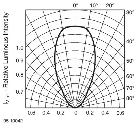
Fig. 3 - Relative Luminous Intensity vs. Angular Displacement
