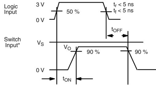
Note: Logic input waveform is inverted for switches that have the opposite logic sense control
