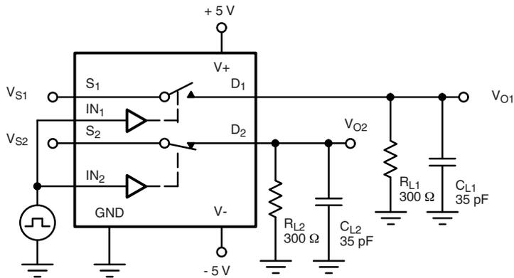
$C_L$  (includes fixture and stray capacitance)
