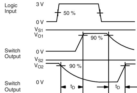
Figure 2. Break-Before-Make (DG613A)
