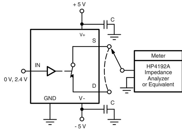
Figure 6. Source/Drain Capacitances
