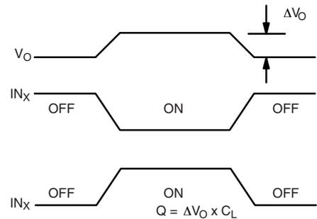
Figure 3. Charge Injection
