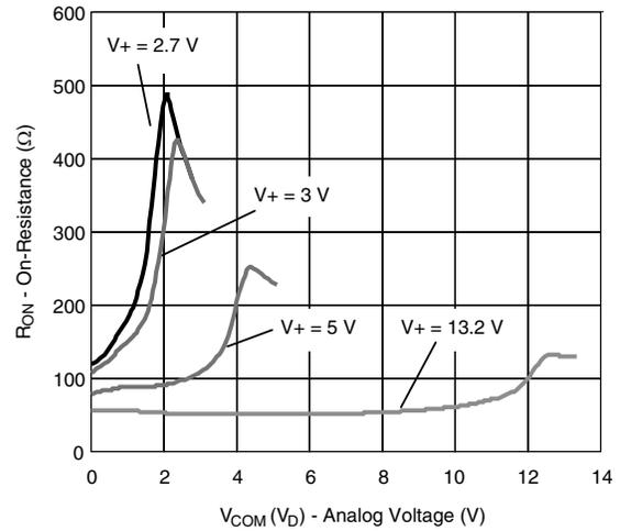
**On-Resistance vs. V<sub>D</sub> (Single Supply)**
