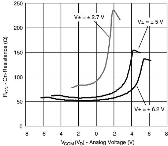
**On-Resistance vs. V<sub>D</sub> (Dual Supply)**
