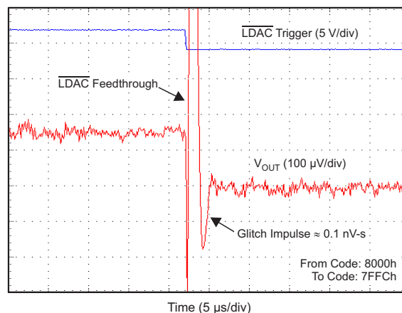
Figure 80. Glitch Impulse, Falling Edge, 1-LSB Step
