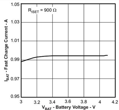
**Figure 11. Fastcharge Current vs Battery Voltage**
