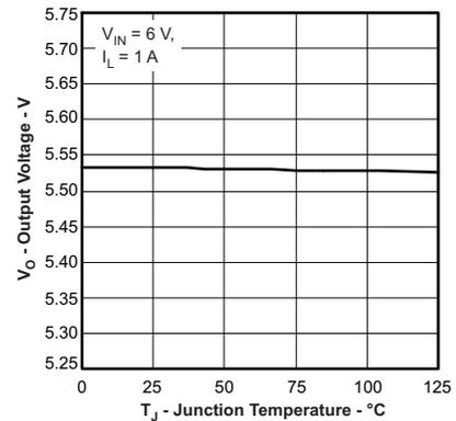
Figure 6. Output Regulation Voltage vs Temperature
