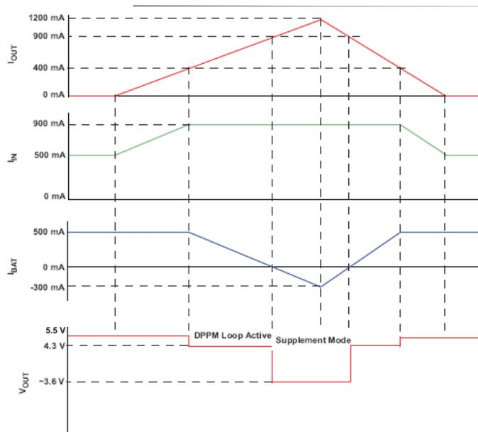
**Figure 21. bq24075T, '79T DPPM and Battery Supplement Modes
