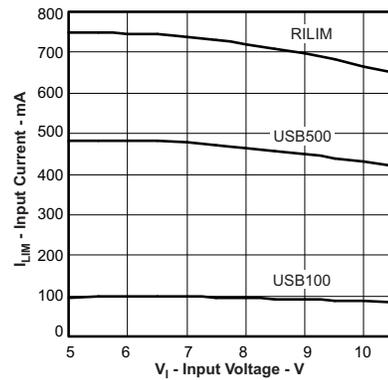
**Figure 10. Input Current Limit vs Input Voltage**
