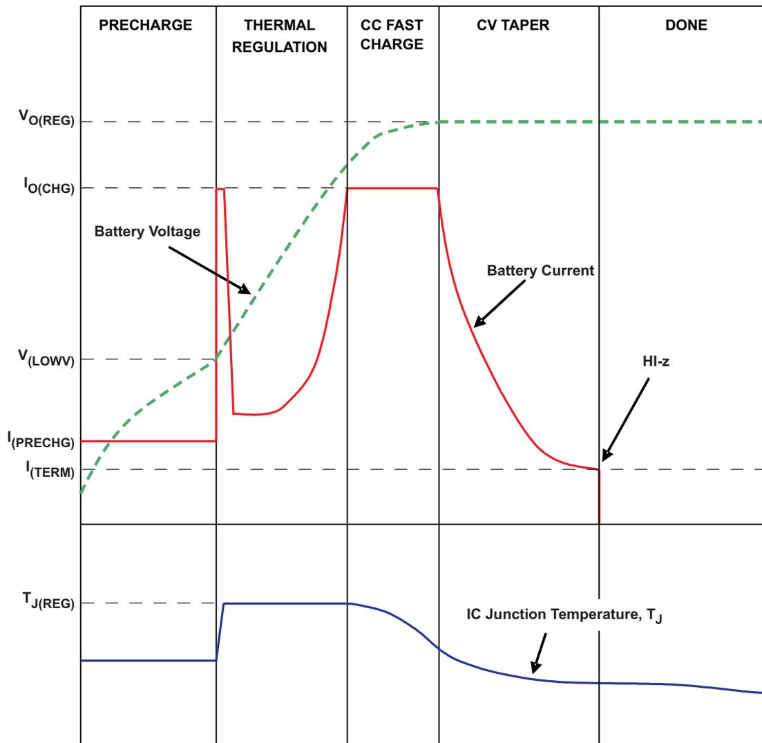
Figure 17. Charge Cycle Modified by Thermal Loop
