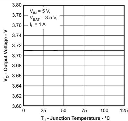
Figure 5. bq24072T Output Regulation Voltage vs Temperature
