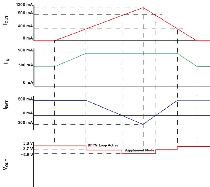
**Figure 22. bq24072T DPPM and Battery Supplement Modes
