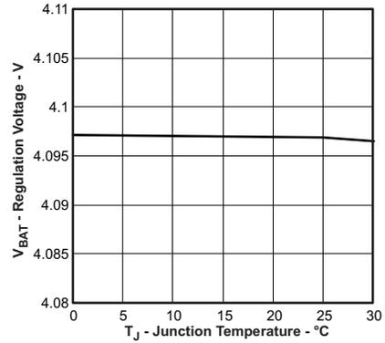
**Figure 8. bq24079T Battery Regulation Voltage vs Temperature**
