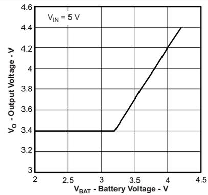
Figure 4. bq24072T Output Regulation Voltage vs Battery Voltage
