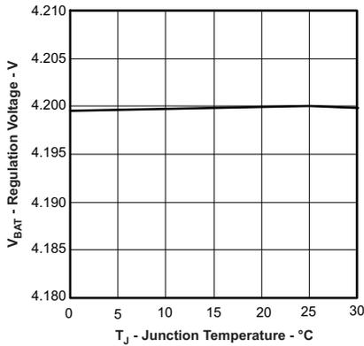
**Figure 7. bq24075T BAT Regulation Voltage vs Temperature**
