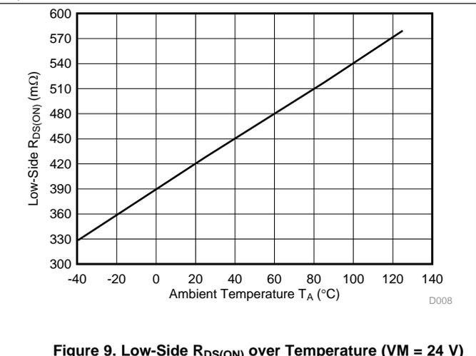
Figure 9. Low-Side  $R_{DS(ON)}$  over Temperature ( $V_M = 24\text{ V}$ )
