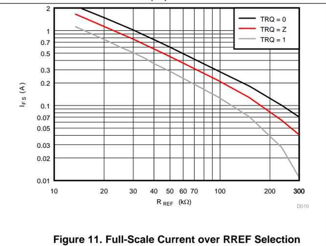
Figure 11. Full-Scale Current over  $R_{REF}$  Selection
