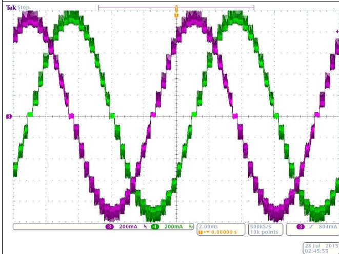
Figure 29. Microstepping Using Mixed 30% Fast Decay on Increasing and Decreasing Steps
