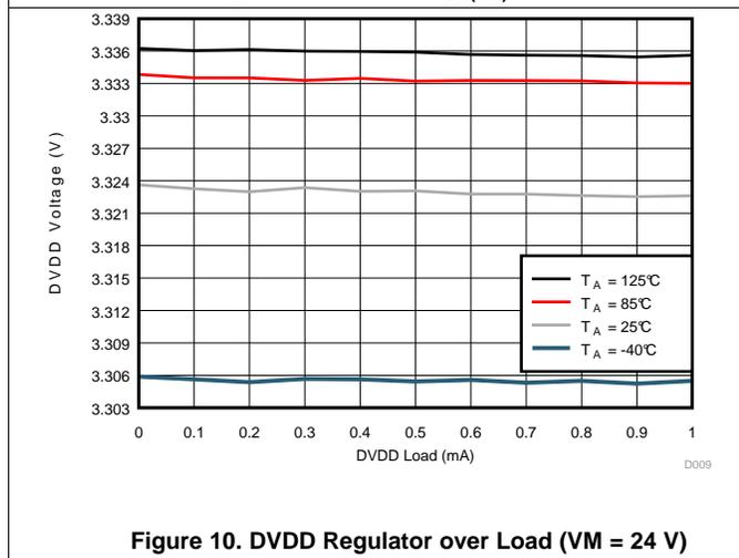
Figure 10. DVDD Regulator over Load ( $V_M = 24\text{ V}$ )
