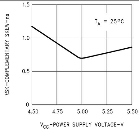
Figure 8. Complementary Skew vs Power Supply Voltage
