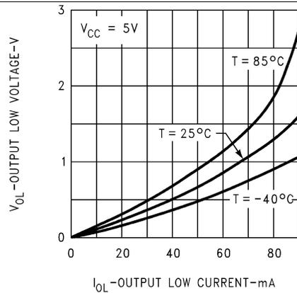
Figure 16. Output Low Voltage vs Output Low Current
