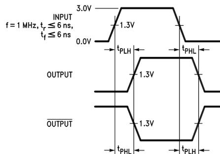
Figure 23. Propagation Delays
