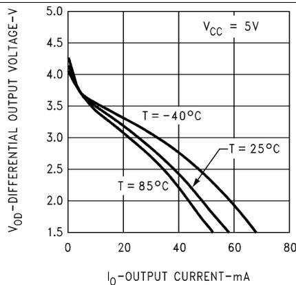
Figure 9. Differential Output Voltage vs Output Current
