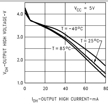
Figure 11. Output High Voltage vs Output High Current
