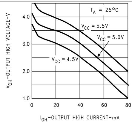
Figure 12. Output High Voltage vs Output High Current
