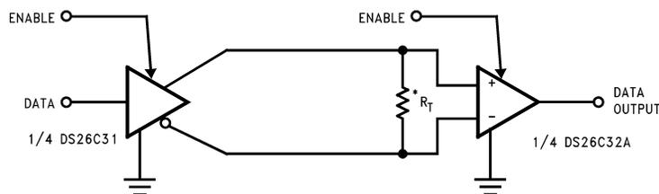
\*R<sub>T</sub> is optional although highly recommended to reduce reflection.
