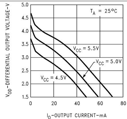
Figure 10. Differential Output Voltage vs Output Current
