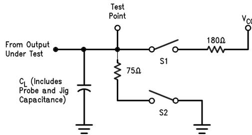
**Figure 26. Load AC Test Circuit for “LS-Type” Load**
