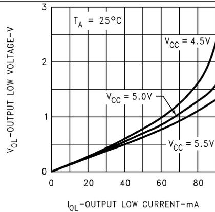
Figure 14. Output Low Voltage vs Output Low Current
