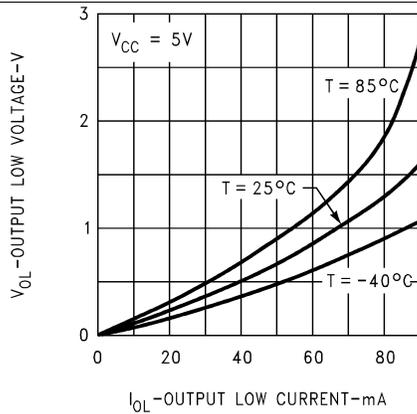
Figure 13. Output Low Voltage vs Output Low Current
