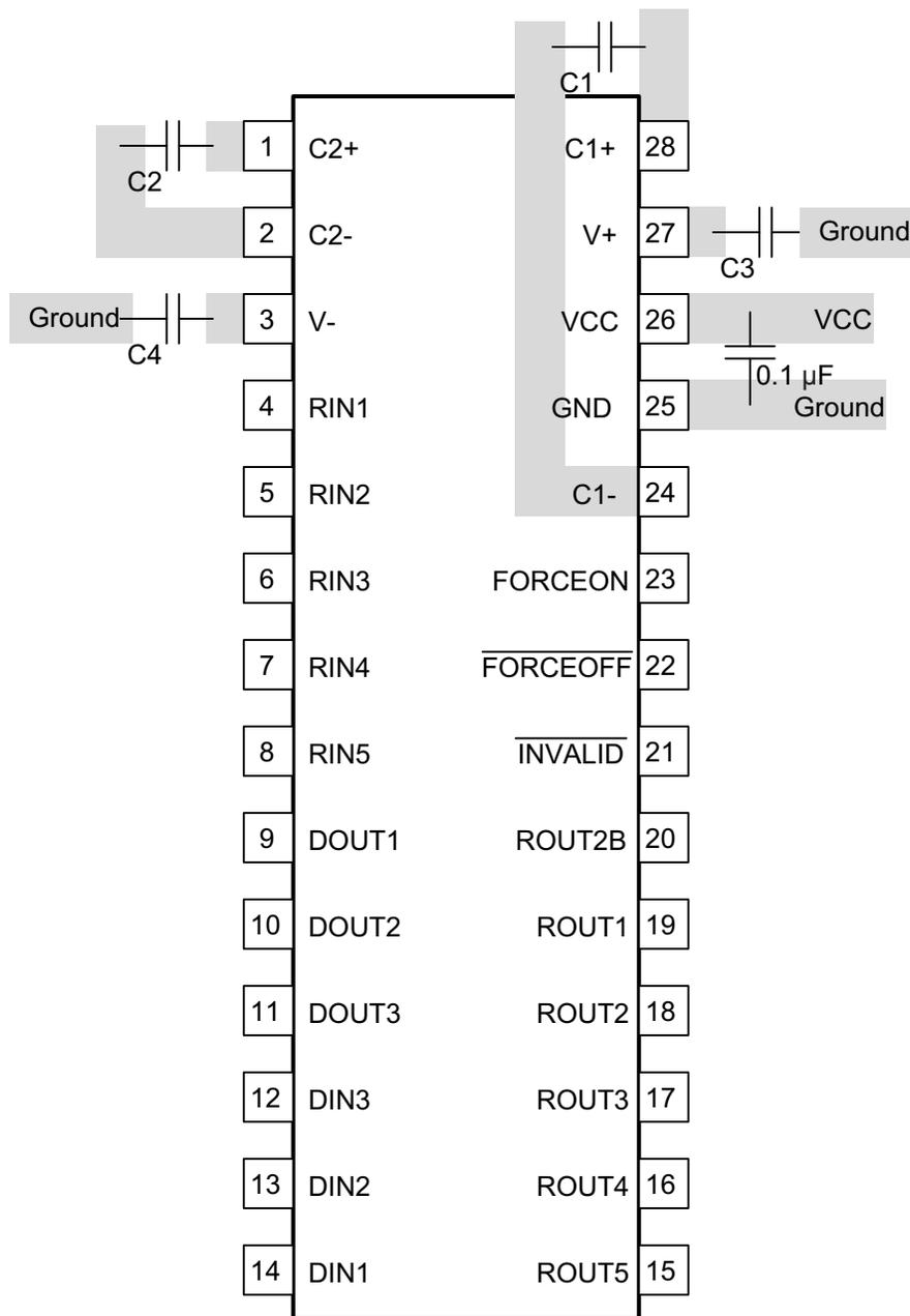
Figure 10. Layout Diagram
