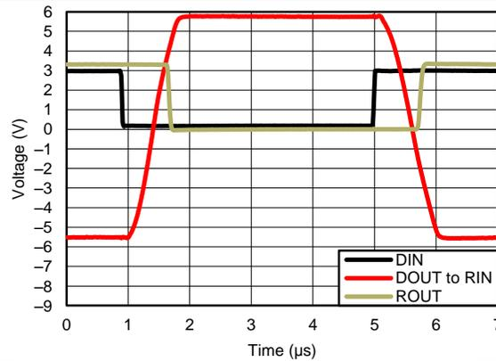
**Figure 9. Driver to Receiver Loopback Timing Waveform**
