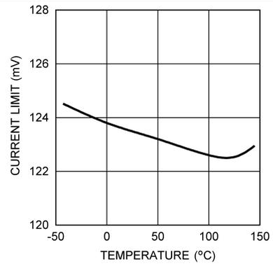
Figure 10. Current-Limit vs Temperature
