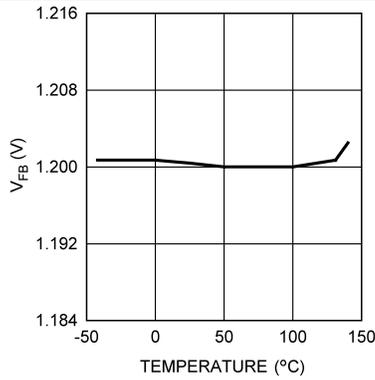
Figure 7. V<sub>FB</sub> vs Temperature
