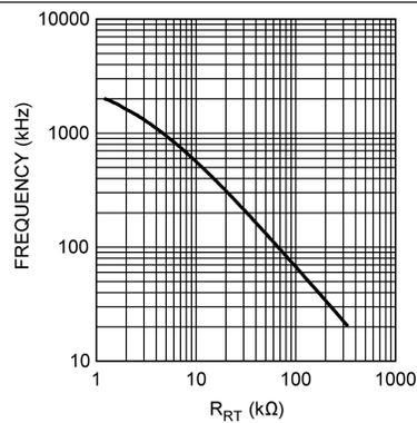
Figure 5. Frequency vs R<sub>RT</sub>
