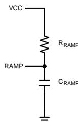
**Figure 23. Additional Slope Compensation for  $V_{OUT} > 5V$**
