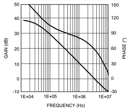
Figure 12. Error Amplifier Gain/Phase
