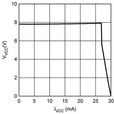
Figure 3. V<sub>CC</sub> vs I<sub>VCC</sub>
