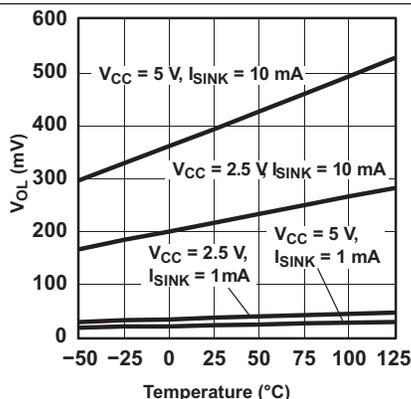
Figure 7. I/O Output Low Voltage vs Temperature
