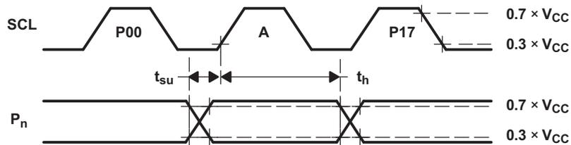
Figure 14. P-Port Load Circuits and Voltage Waveforms
