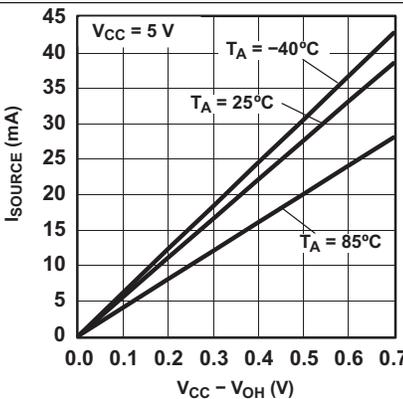
Figure 10. I/O Source Current vs Output High Voltage
