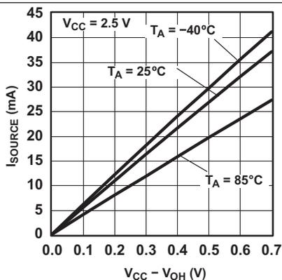
Figure 8. I/O Source Current vs Output High Voltage
