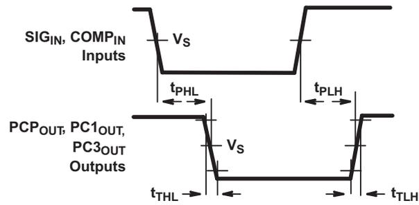
**Figure 4. Input-to-Output Propagation Delays and Output Transition Times**
