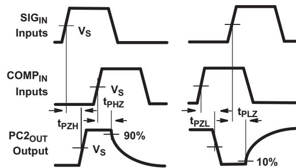
**Figure 5. 3-State Enable and Disable Times for PC2<sub>OUT</sub>**
