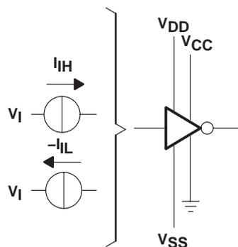
**Figure 2. Driver Test Circuit for I<sub>IH</sub> and I<sub>IL</sub>**
