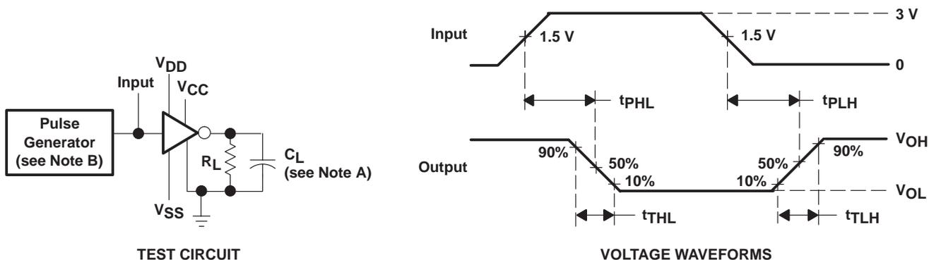
NOTES: A.  $C_L$  includes probe and jig capacitance.
