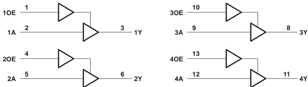
Pin numbers shown are for the D, DB, DGV, J, NS, PW, and W packages.
