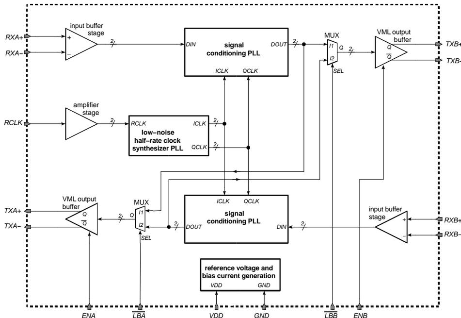
Figure 1. Simplified Block Diagram of the TLK1002A Transceiver
