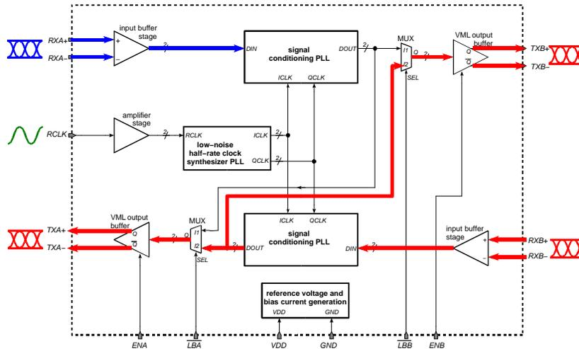
**Figure 6. Data Path in Internal Loop-Back Mode B**
