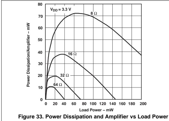
Figure 33. Power Dissipation and Amplifier vs Load Power
