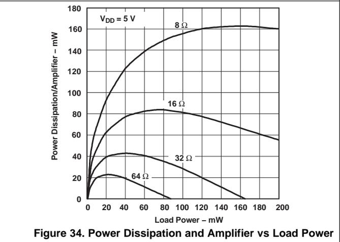
Figure 34. Power Dissipation and Amplifier vs Load Power
