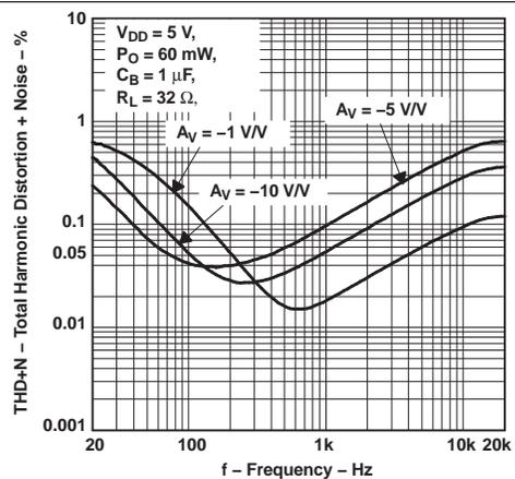
Figure 3. Total Harmonic Distortion + Noise vs Frequency
