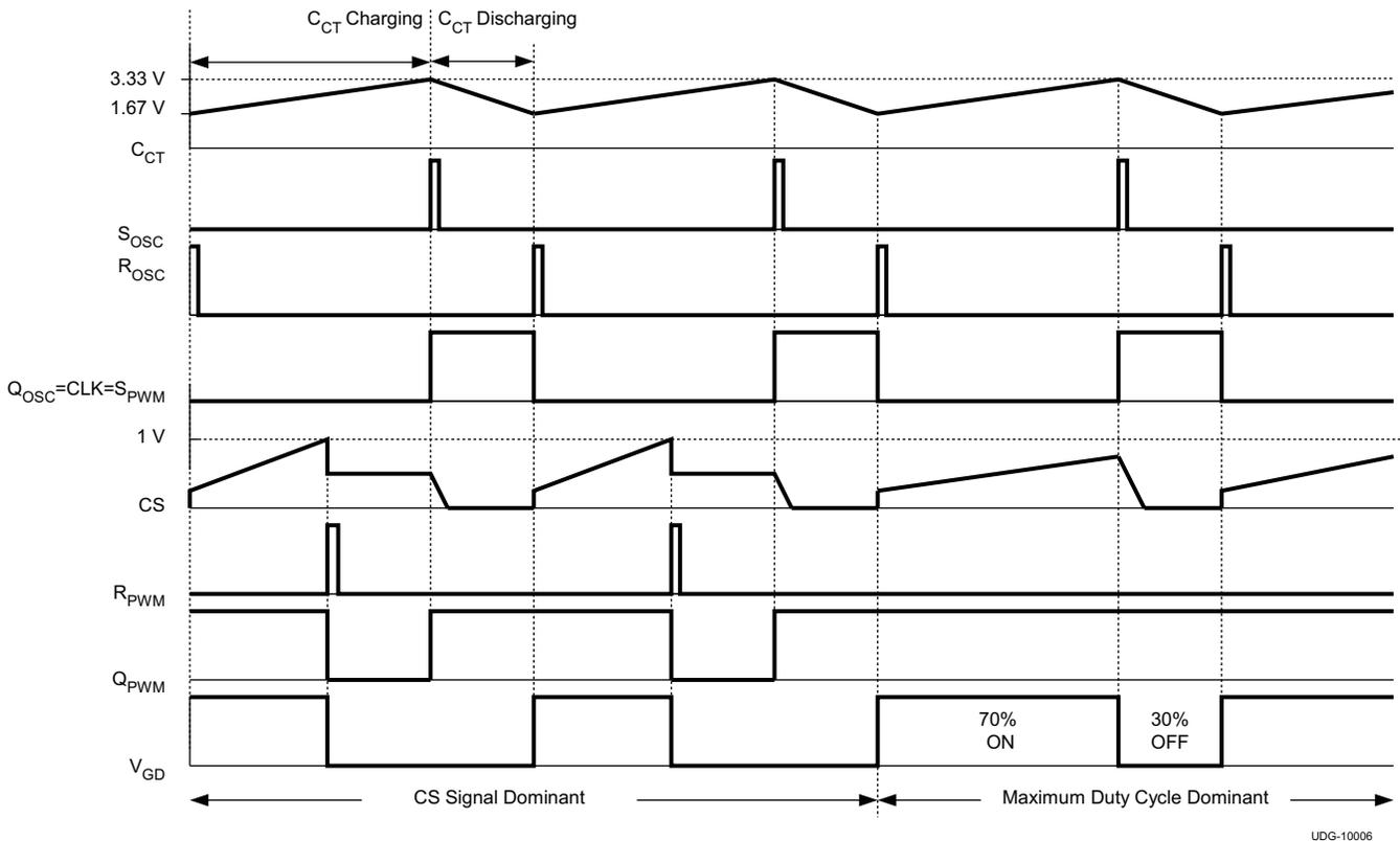
Figure 2. Oscillator Latch and PWM Latch Waveforms
