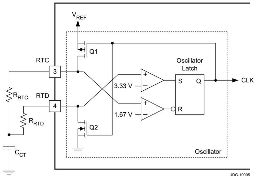
**Figure 1. Oscillator Function**
