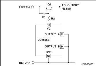
For single-ended supplies, the driver outputs are grounded. The VC terminal is switched to ground by the to-tem-pole source transistors on alternate oscillator cycles.
