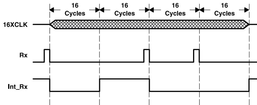
Figure 36. Positive Rx Pulse Decode – Macro View
