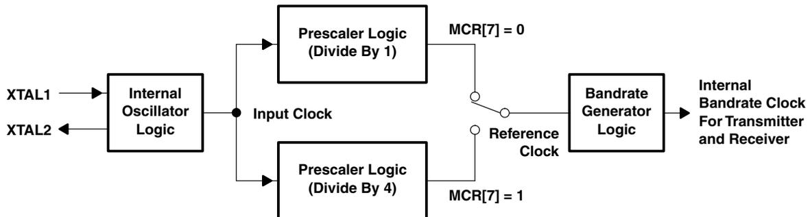
Figure 9. Prescaler and Baud Rate Generator Block Diagram
