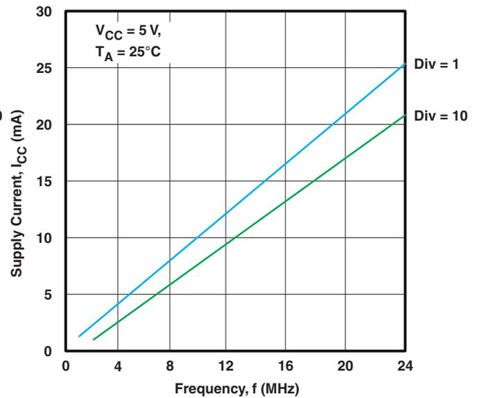
Figure 14. Supply Current vs Frequency ( $V_{CC} = 5\text{ V}$ )
