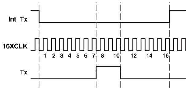
Figure 29. IrDA-SIR Encoding Scheme – Detailed Timing Diagram
