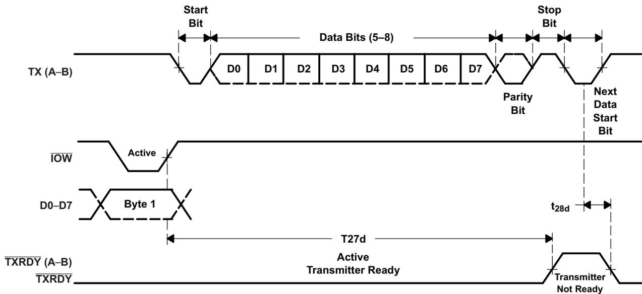
Figure 22. Transmit Ready Timing in None FIFO Mode
