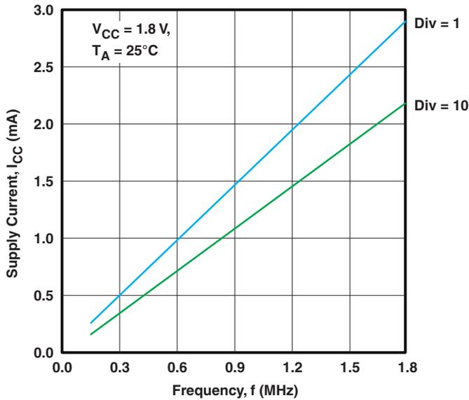
Figure 11. Supply Current vs Frequency ( $V_{CC} = 1.8\text{ V}$ )
