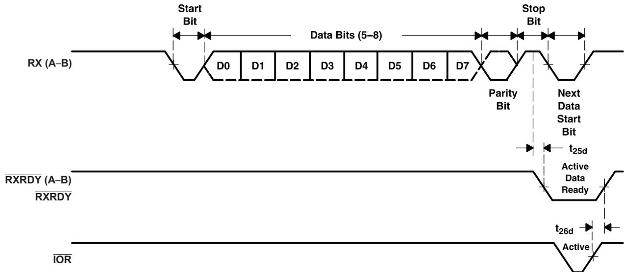
Figure 19. Receive Ready Timing in Non-FIFO Mode
