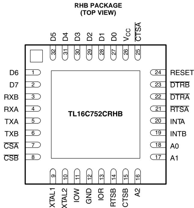
NOTE: The 32-pin RHB package does not provide access to  $\overline{DSRA}$ ,  $\overline{DSRB}$ ,  $\overline{RIA}$ ,  $\overline{RIB}$ ,  $\overline{CDA}$ , and  $\overline{CDB}$  inputs or  $\overline{OPA}$ ,  $\overline{OPB}$ ,  $\overline{RXRDYA}$ ,  $\overline{RXRDYB}$ , and  $\overline{TXRDYA}$  outputs.
