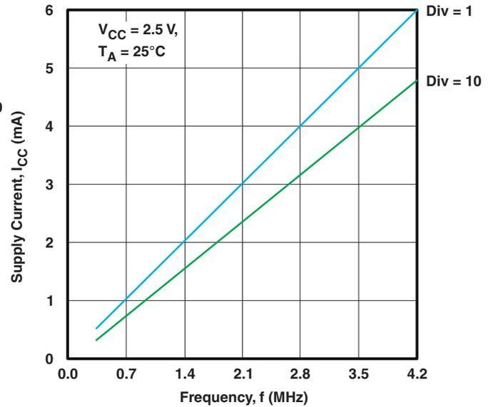
Figure 12. Supply Current vs Frequency ( $V_{CC} = 2.5\text{ V}$ )
