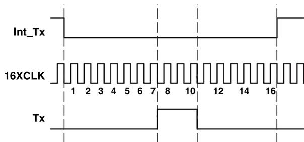
Figure 31. IrDA-SIR Decoding Scheme – Detailed Timing Diagram
