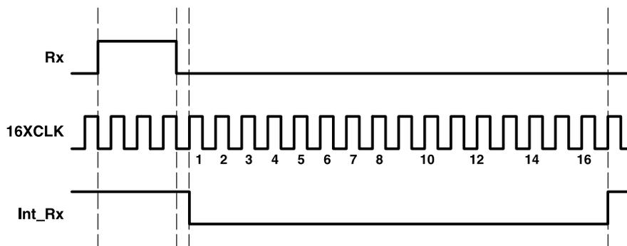
Figure 35. Positive Rx Pulse Decode – Detailed View
