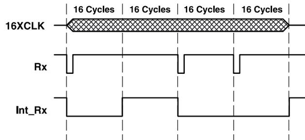
Figure 32. IrDA-SIR Decoding Scheme – Macro View
