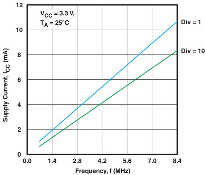
Figure 13. Supply Current vs Frequency ( $V_{CC} = 3.3\text{ V}$ )
