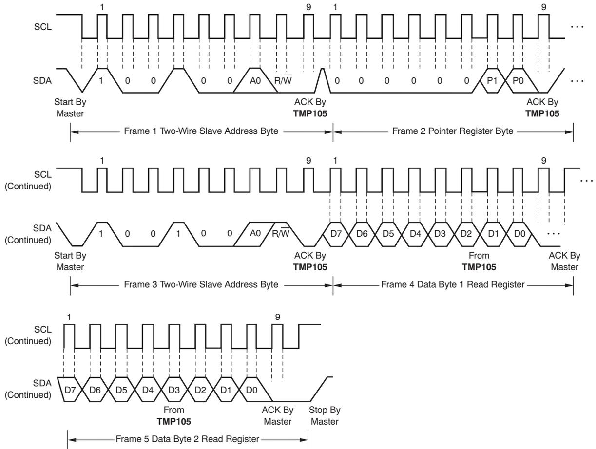
Figure 6. Two-Wire Timing Diagram for Read Word Format
