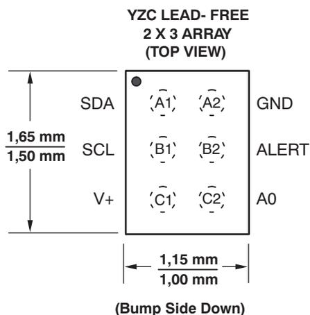
Note: Pin A1 is marked with a 0 for Pb-free (YZC)
