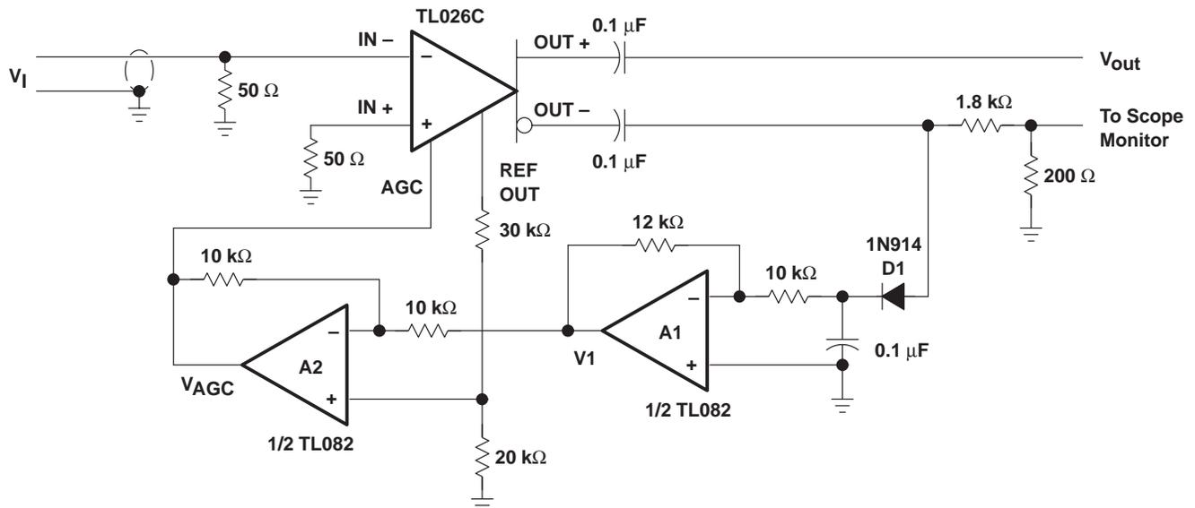
NOTE:  $V_{CC+} = 6\text{ V}$  and  $V_{CC-} = -6\text{ V}$  for TL026C and amplifiers A1 and A2.
