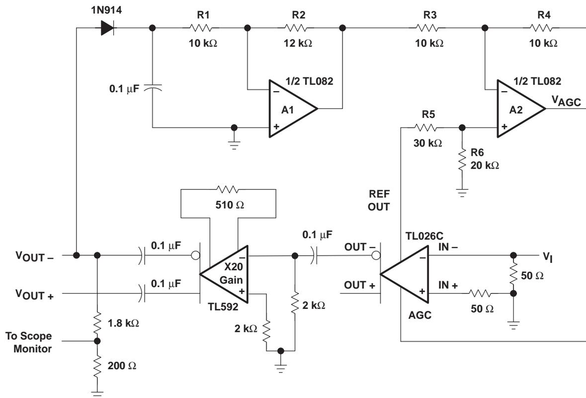
NOTE:  $V_{CC+} = 6\text{ V}$  and  $V_{CC-} = -6\text{ V}$  for TL026C and amplifiers A1 and A2.
