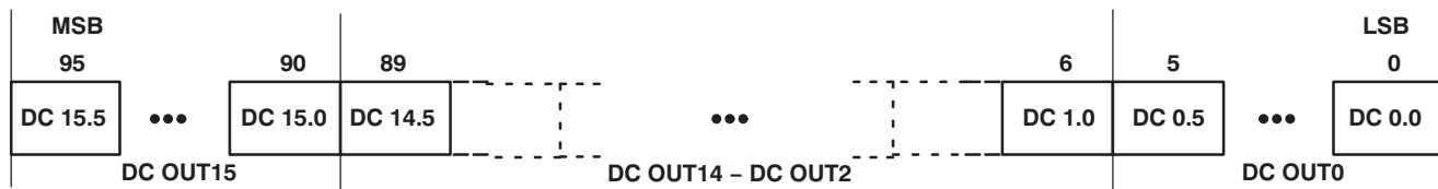
Figure 15. Dot Correction Data Packet Format
