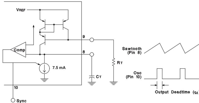
Output deadtime is determined by the external capacitor,  $C_T$ , according to the formula:
