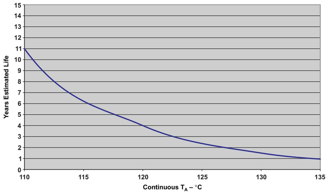
Figure 1. UC1846MDWREP Estimated Device Life at Elevated Temperatures
