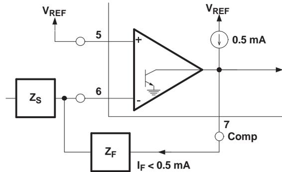
Error amplifier can source up to 0.5 mA.
