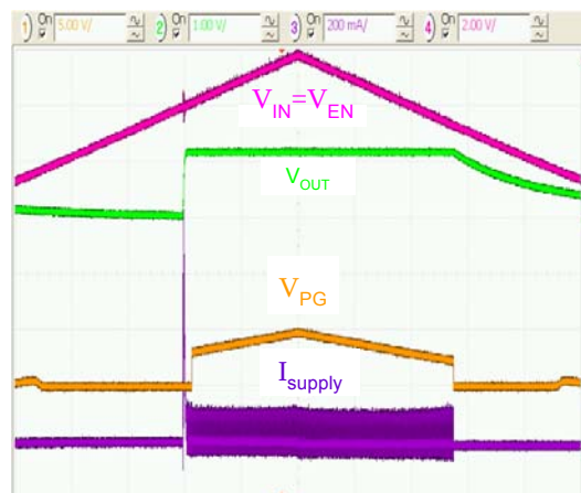
Figure 18. Soft-Start, EN Pin Tied to VCC I_{LOAD}=0 , 1 ms/div.
