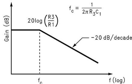
Figure 42. Frequency Response of Simple Low-pass Active Filter
