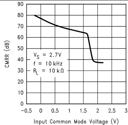
Figure 14. CMRR vs Input Common Mode Voltage
