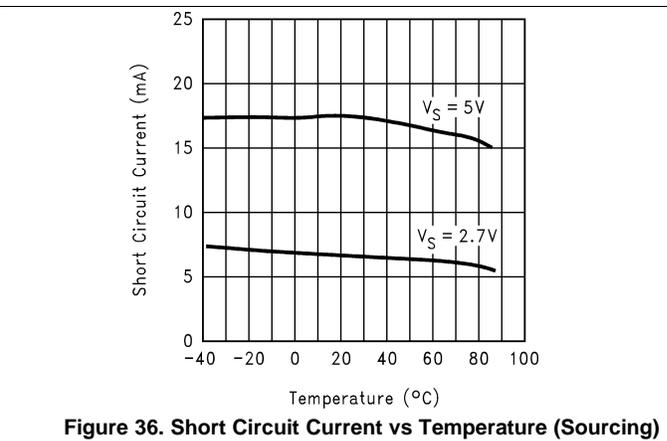
Figure 36. Short Circuit Current vs Temperature (Sourcing)
