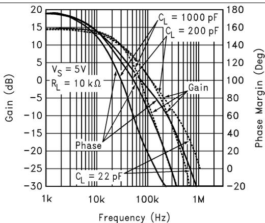
Figure 23. Gain and Phase vs Capacitive Load
