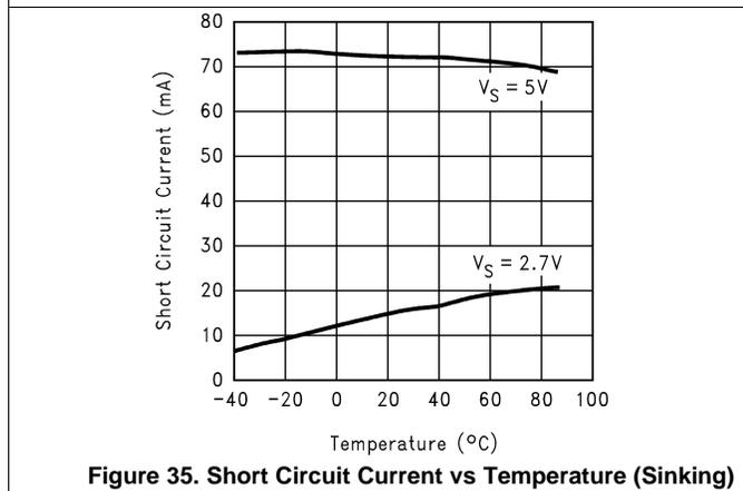
Figure 35. Short Circuit Current vs Temperature (Sinking)
