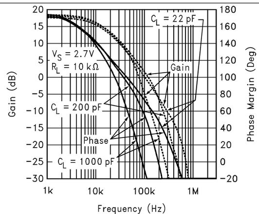
Figure 22. Gain and Phase vs Capacitive Load
