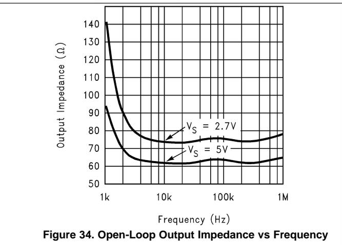
Figure 34. Open-Loop Output Impedance vs Frequency
