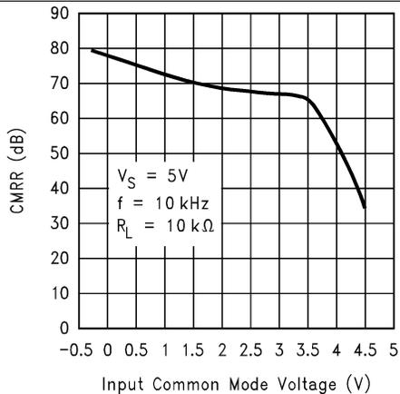
Figure 15. CMRR vs Input Common Mode Voltage
