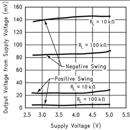
Figure 7. Output Voltage Swing vs Supply Voltage
