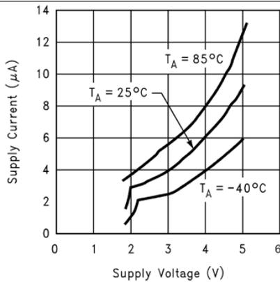
Figure 1. Supply Current vs Supply Voltage (LPV321-N)
