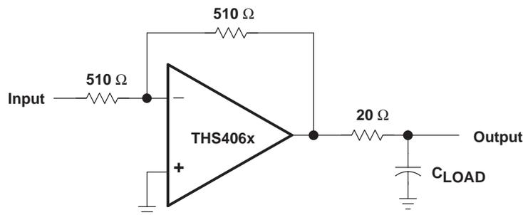
Figure 28. Driving a Capacitive Load
