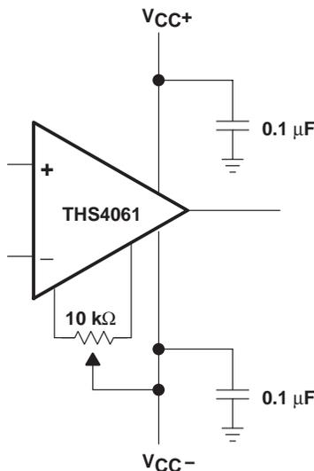
Figure 26. Offset Nulling Schematic
