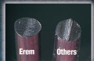
Erem Full Flush and Super Full Flush cutters leave a flat surface on cut leads.
