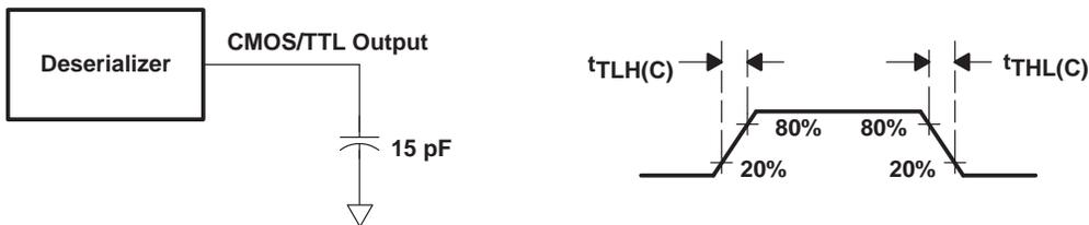
**Figure 5. Deserializer CMOS/TTL Output Load and Transition Times**
