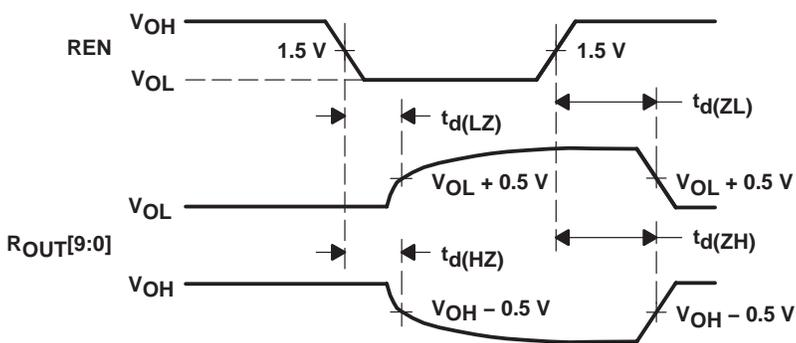
Figure 14. Deserializer High-Impedance-State Test Circuit and Timing
