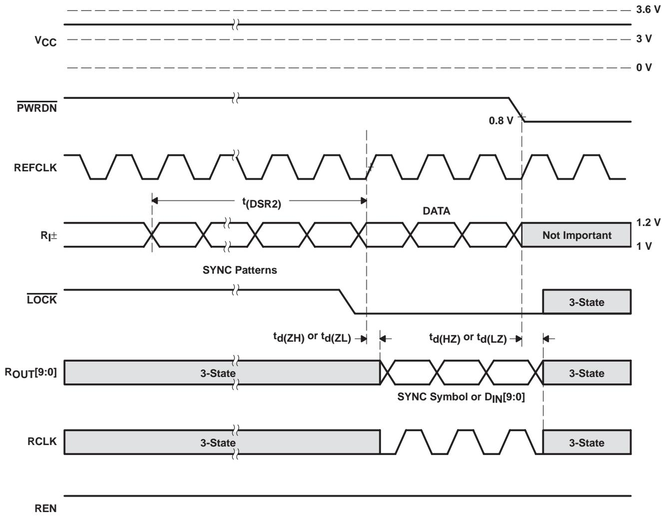
Figure 16. Deserilaizer PLL Lock Time From SyncPAT
