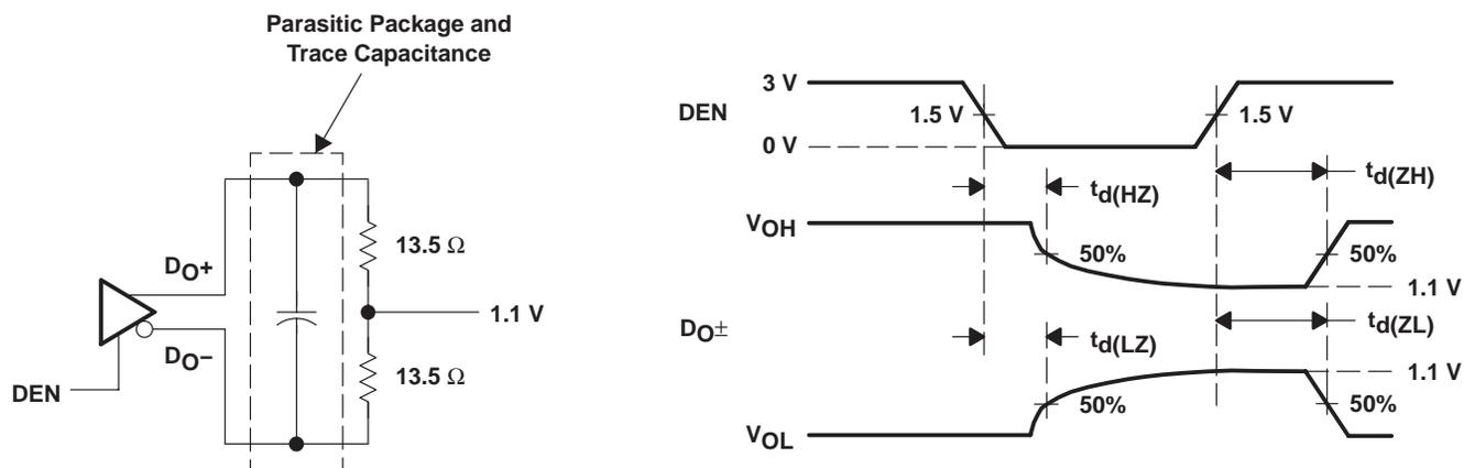
Figure 8. Serializer High-Impedance-State Test Circuit and Timing
