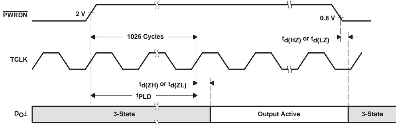
Figure 9. Serializer PLL Lock Time and  $\overline{PWRDN}$  High-Impedance-State Delays
