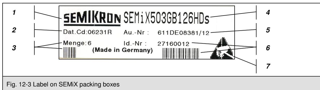
Fig. 12-3 Label on SEMiX packing boxes
