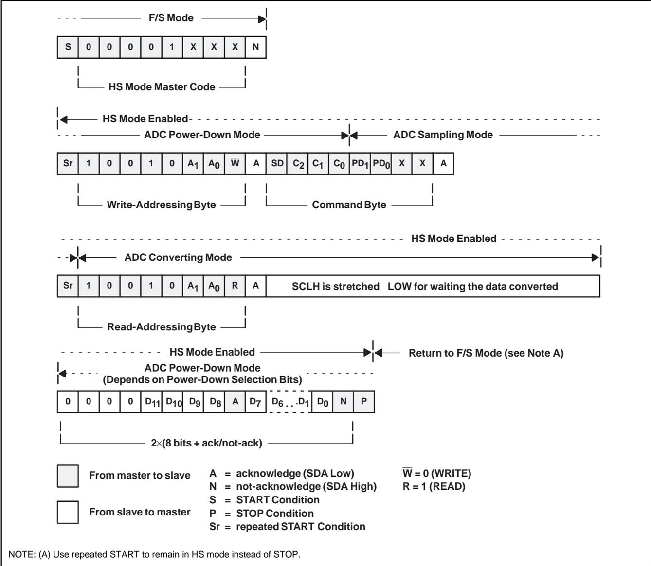
FIGURE 4. Typical Read Sequence in HS Mode.
