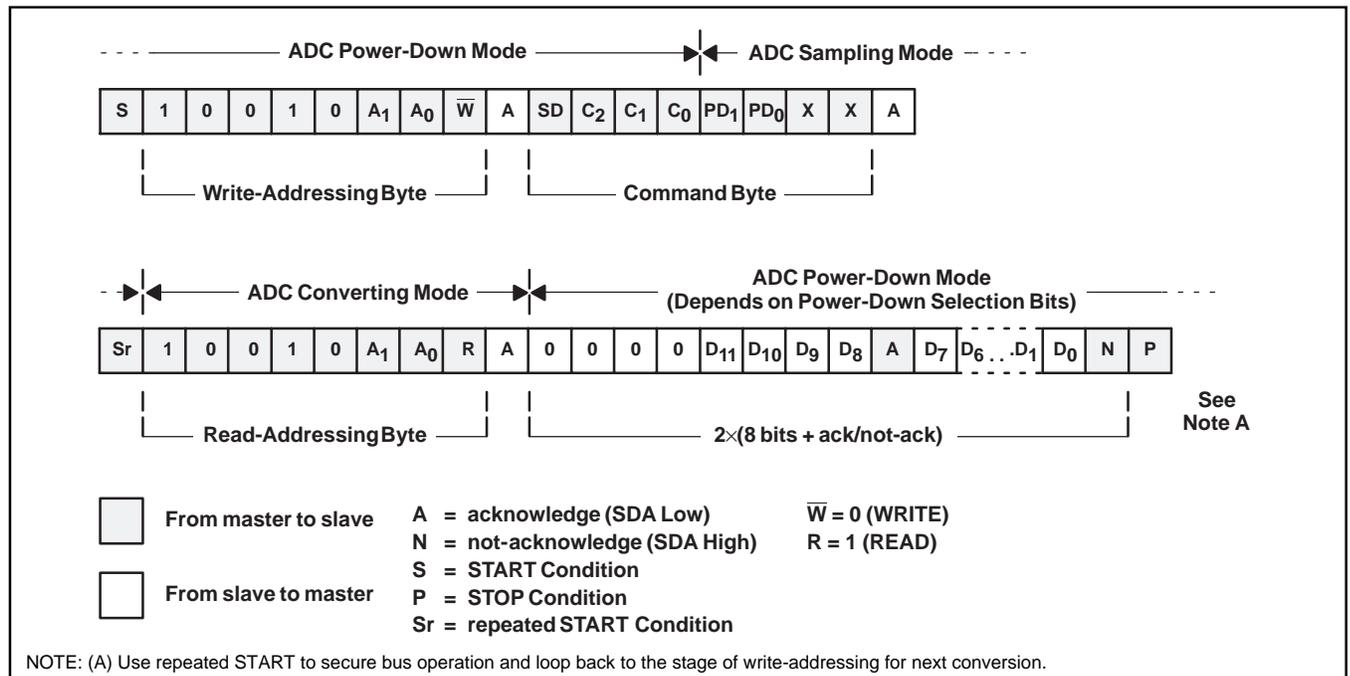
FIGURE 3. Typical Read Sequence in F/S Mode.
