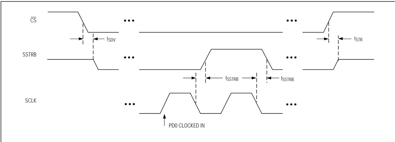
Figure 8. External Clock Mode SSTRB Detailed Timing
