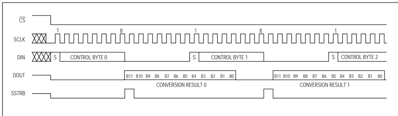
Figure 11a. External Clock Mode, 15 Clocks/Conversion Timing
