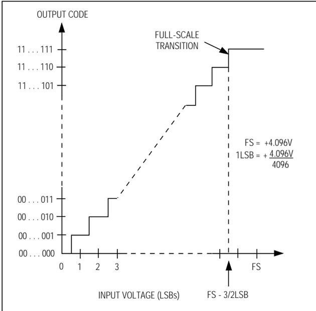
Figure 15. Unipolar Transfer Function,  $4.096V = \text{Full Scale}$
