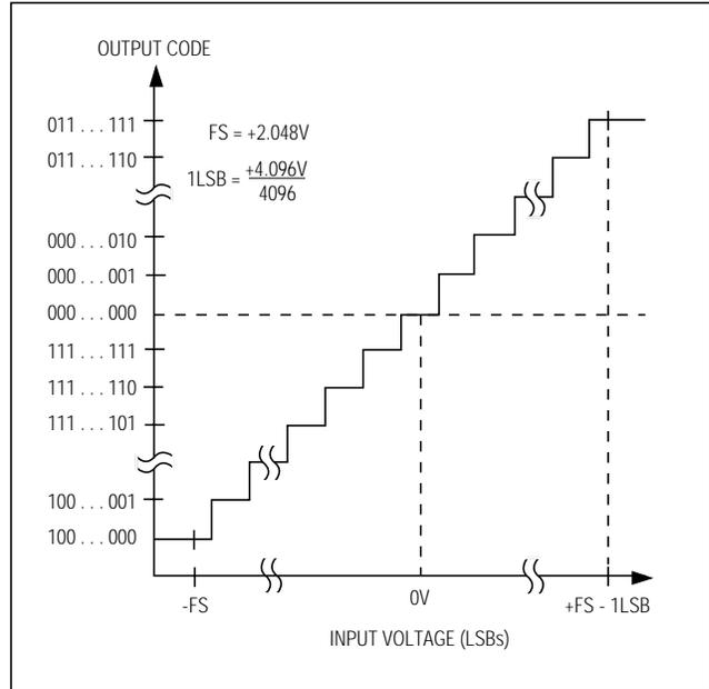
Figure 16. Bipolar Transfer Function,  $\pm 4.096V/2 = \text{Full Scale}$
