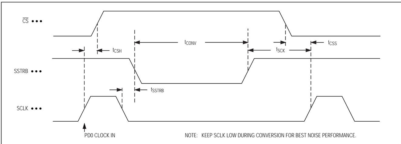
Figure 10. Internal Clock Mode SSTRB Detailed Timing
