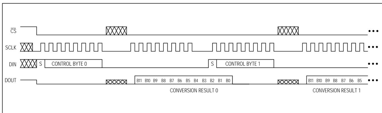
Figure 11b. External Clock Mode, 16 Clocks/Conversion Timing
