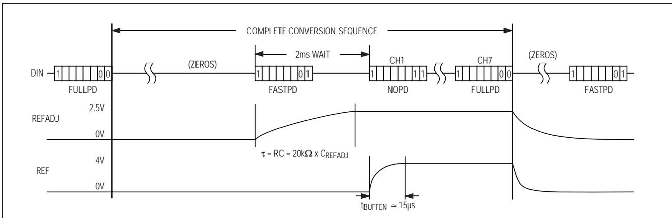
Figure 13. MAX1202 FULLLPD/FASTPD Power-Up Sequence
