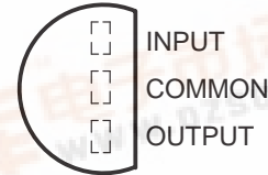
LP PACKAGE (TO-92, TO-226AA) (TOP VIEW)
