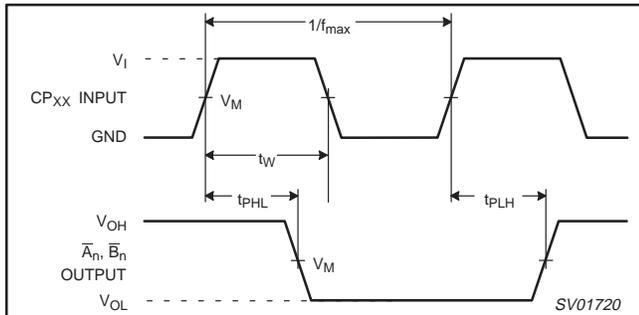
**Figure 1. Clock input ( $CP_{BA}$ ,  $CP_{AB}$ ) to output ( $\overline{B}_n$ ,  $\overline{A}_n$ ) propagation delays, the clock pulse width and the maximum clock frequency.**
