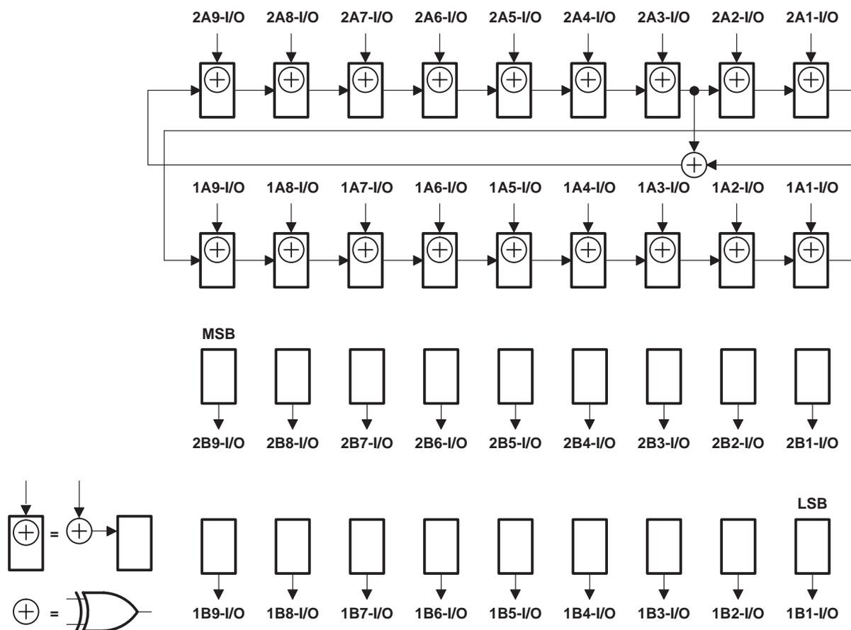
Figure 11. 18-Bit PSA/COUNT Configuration ( $\overline{1OEAB} = \overline{2OEAB} = 0$ ,  $\overline{1OEB\bar{A}} = \overline{2OEB\bar{A}} = 1$ )
