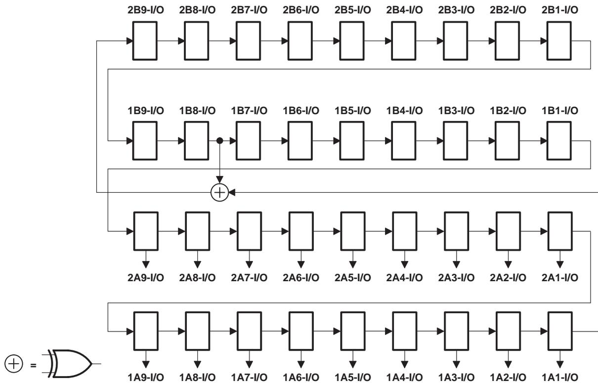
**Figure 6. 36-Bit PRPG Configuration ( $\overline{1OEAB} = \overline{2OEAB} = 1$ ,  $\overline{1OEBA} = \overline{2OEBA} = 0$ )**
