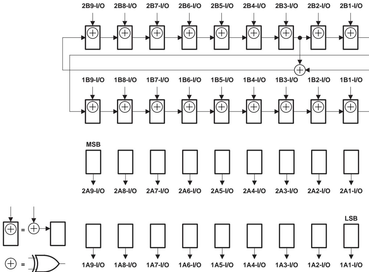
Figure 12. 18-Bit PSA/COUNT Configuration ( $\overline{1OEAB} = \overline{2OEAB} = 1$ ,  $\overline{1OEBA} = \overline{2OEBA} = 0$ )
