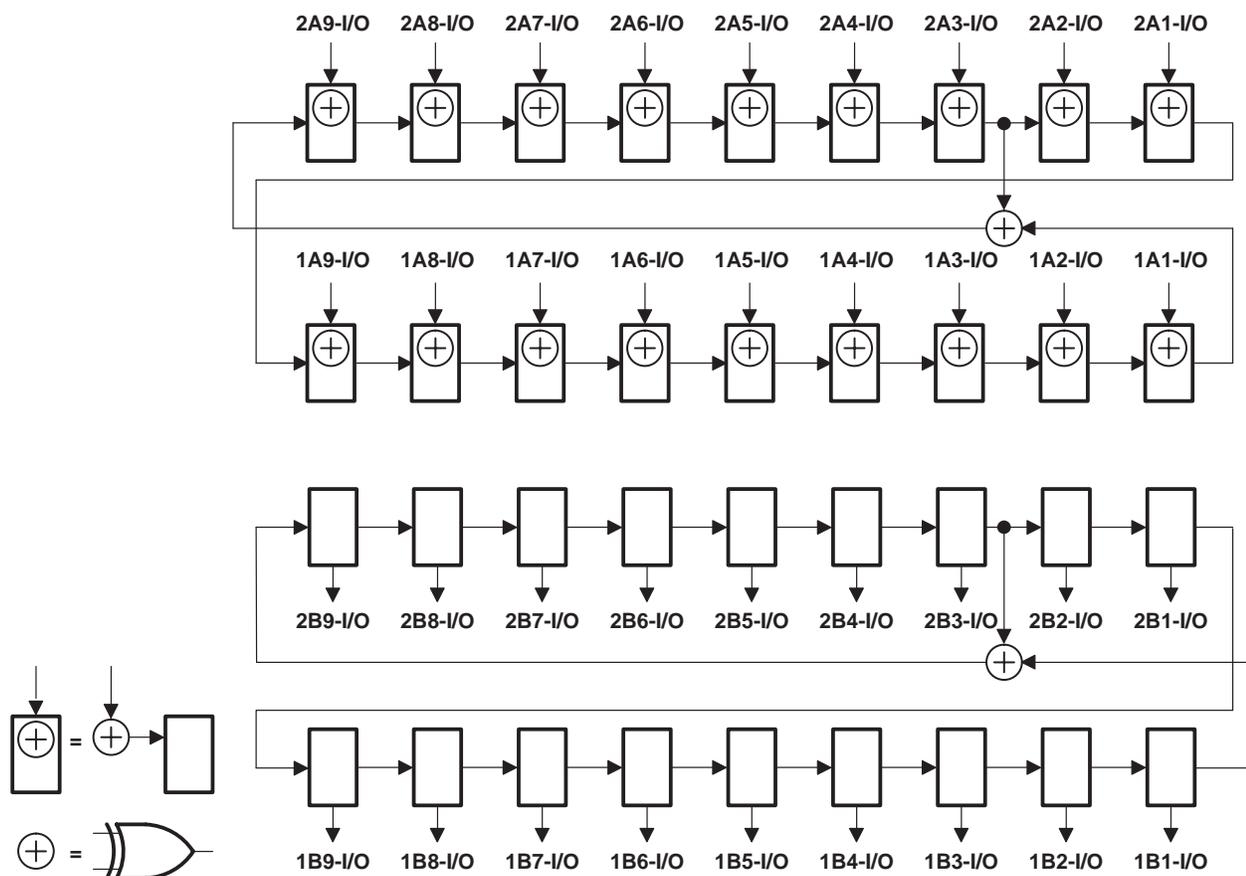
Figure 9. 18-Bit PSA/PRPG Configuration ( $\overline{1OEAB} = \overline{2OEAB} = 0$ ,  $\overline{1OEBA} = \overline{2OEBA} = 1$ )
