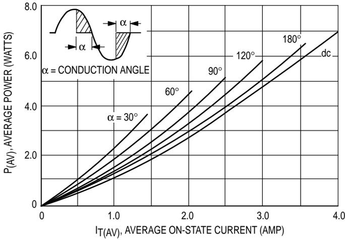
**FIGURE 4 – POWER DISSIPATION**
