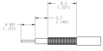
RECOMMENDED CABLE STRIPPING DIM'S. SCALE 3.000
