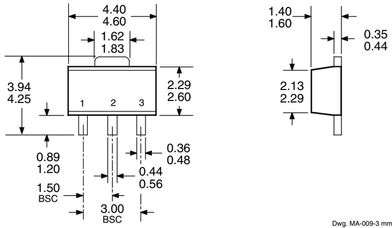
NOTE: Exact body and lead configuration at vendor's option within limits shown.
