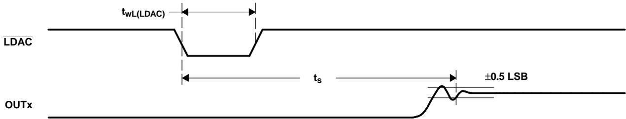
**Figure 12. Output Timing**
