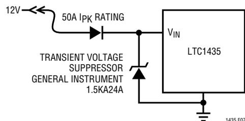
Figure 7. Automotive Application Protection
